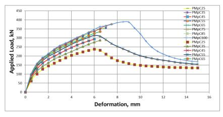
Fig. 20. Effect of column size on load deformation diagram
