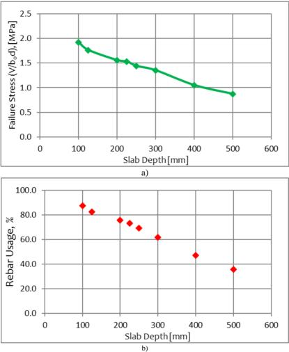
Fig. 9. Effect of slab depth on: a) failure stress b) percentage reinforcement utilization
