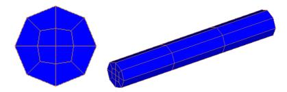
Fig. 2. Hexahedron mesh of steel
