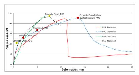
Fig. 5. Load deformation diagram of experimental and numerical modeling of PG6 & PM2
