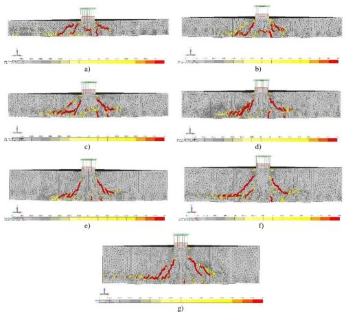
Fig. 10. Progress of crack pattern with depth for: a) 100mm slab depth, b) 125mm slab depth, c) 200mm slab depth d) 225mm slab depth, e) 300mm slab depth, f) 400mm slab depth and g) 500mm slab depth
