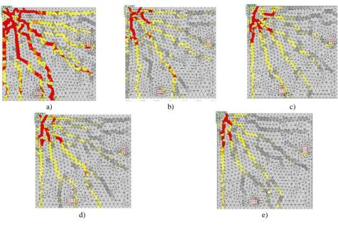
Fig. 19. Flexural crack pattern on tension side of the slab at failure (a)  $\rho=0.49$ , (b)  $\rho=0.8$ , (c)  $\rho=1.0$ , (d)  $\rho=1.5$ , (e)  $\rho=2.0$
