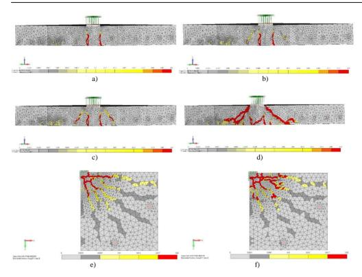
Fig. 4. Specimen PG6 crack propagation: a) flexural crack; b) onset of shear crack; c) crack at peak load;d) Post punching crack; e) plan view of flexural crack at peak load;f) plan view of flexural crack after punching failure at ultimate load
