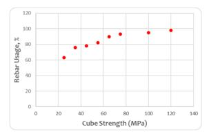
Fig. 14. Percentage utilization of flexural reinforcement
