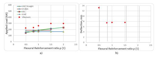
Fig. 15. The effect of dowel action on: a) failure load; b) peak load deformation (add discussion)
