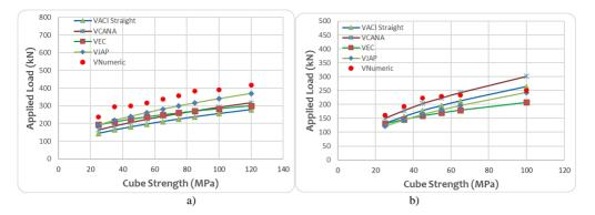
**Fig. 11.** The effect of concrete grade on punching strength: a) adequately reinforced slab ( $\rho$ =1,5); b) lightly reinforced slab ( $\rho$ =0,49)
