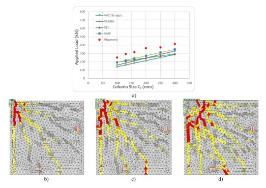
Fig. 21. The effect of column size on: a) Peak Load; c-d) crack pattern [b) C=100mm, c) C=160mm, d) C=300mm]
