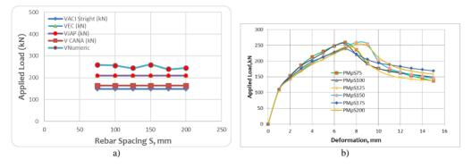
Fig. 22. The effect of Reinforcement spacing on punching shear strength: a) Load Deformation diagram; b) effect of spacing on peak load
