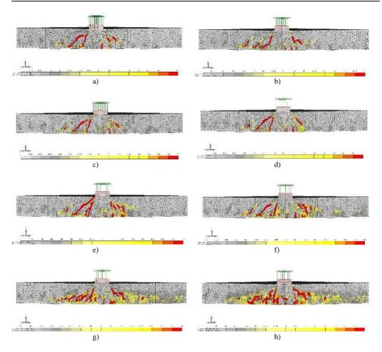
Fig. 13. Crack pattern at failure load for concrete grade of a) C-25 b) C-35 c) C-45 d) C-55 e) C-65 f) C-75 g) C-85 h) C-100
