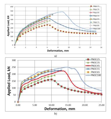
**Fig. 12.** The effect of concrete grade on Load deformation diagram: a) adequately reinforced slab ( $\rho$ =1,5); b) lightly reinforced slab ( $\rho$ =0, 49)
