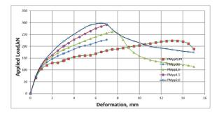
Fig. 16. The effect of flexural reinforcement on load deformation diagram
