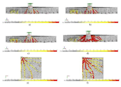
Fig. 6. Specimen PM2 crack propagation: a) flexure-shear crack at yielding; b) onset of ultimate Rebar stress;
