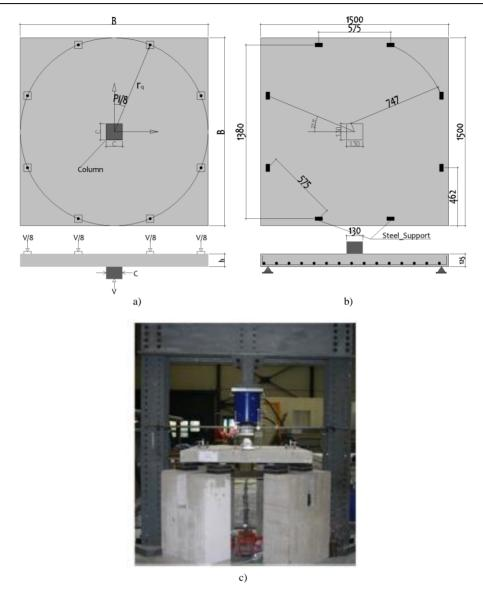
**Fig. 3.** Schematic drawing of slabs used for numerical validation: a) PG6 [19] b) PM2 [20], c) experimental setup of PM2 [20]
