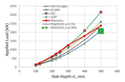
Fig. 7. Effect of Slab depth on punching shear capacity
