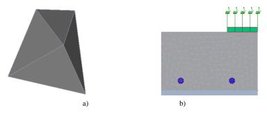
Fig. 1. a) tetrahedron mesh of concrete; b) modeling of steel, concrete and loading plate
