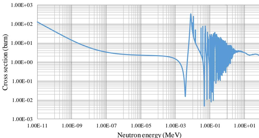
Fig. 4. Neutrons incident energy against displacement damage cross section using iron
