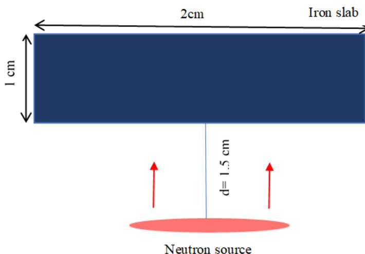
Fig. 2. Schematic diagram showing the slab geometry by a monodirectional neutron source.
