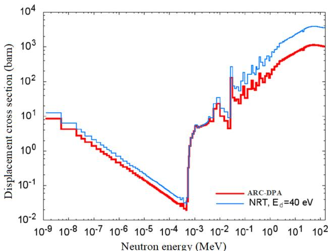
Fig. 1. Displacement cross section against neutron energy for iron
