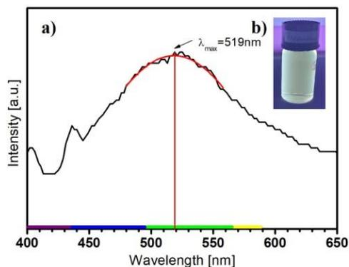
**Fig. 7.** Sample 4: a) photoluminescence emission spectrum, b) sample under UV light
