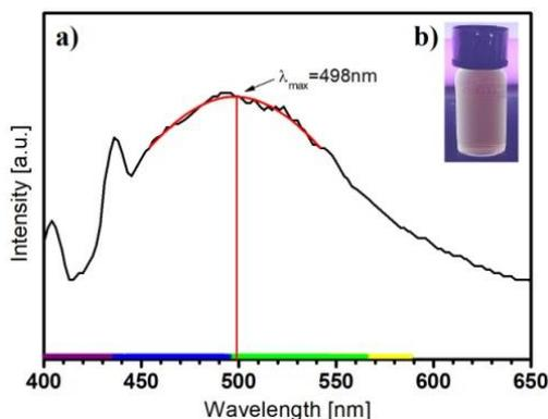
**Fig. 6.** Sample 3: a) photoluminescence emission spectrum, b) sample under UV light
