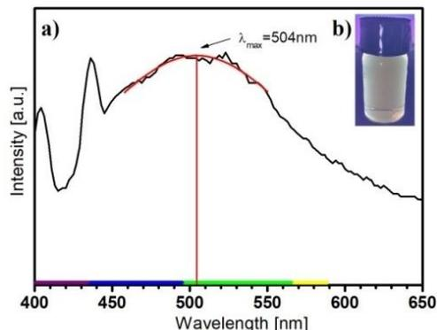
**Fig. 5.** Sample 2: a) photoluminescence emission spectrum, b) sample under UV light
