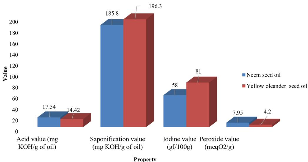
Fig. 4. Chemical Properties of Neem and Yellow Oleander Seed Oils
