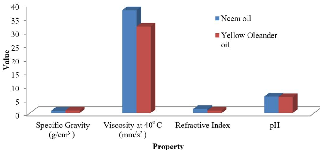
**Fig. 3.** Physical Properties of Neem and Yellow Oleander Seed Oils
