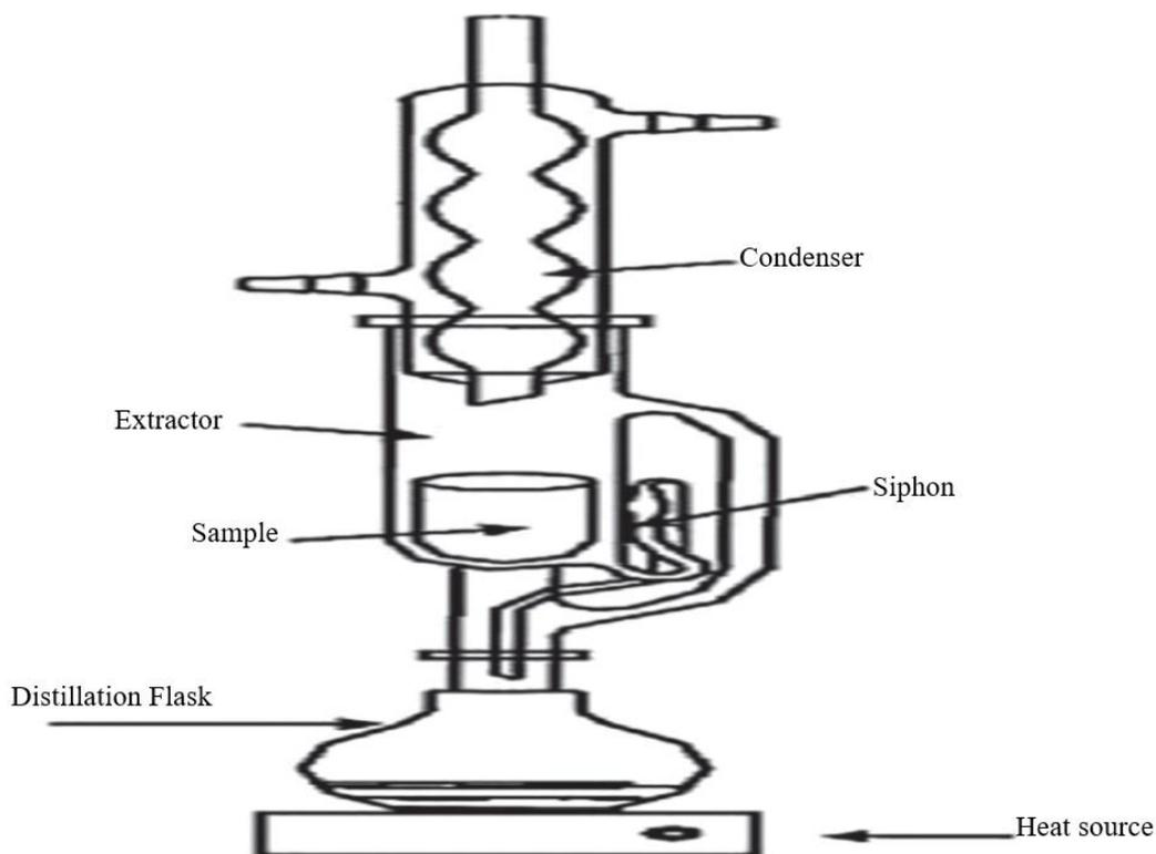
**Fig. 1.** Oil Extraction Set up using Soxhlet Extractor Determination of specific gravity
