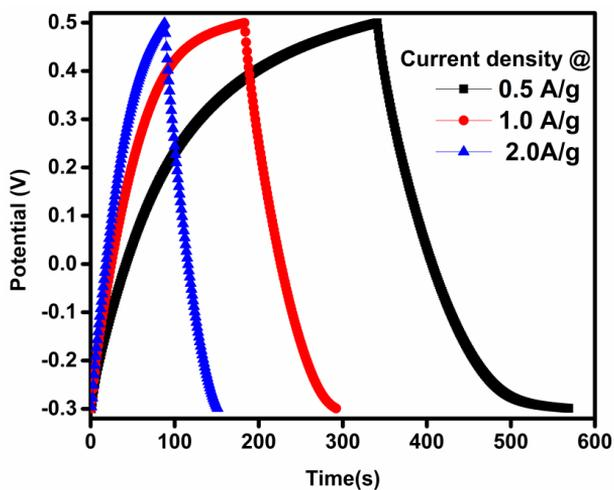
Fig. 8. Galvano static charge–discharge curves of  $\text{Li}_4\text{Ti}_5\text{O}_{12}$
