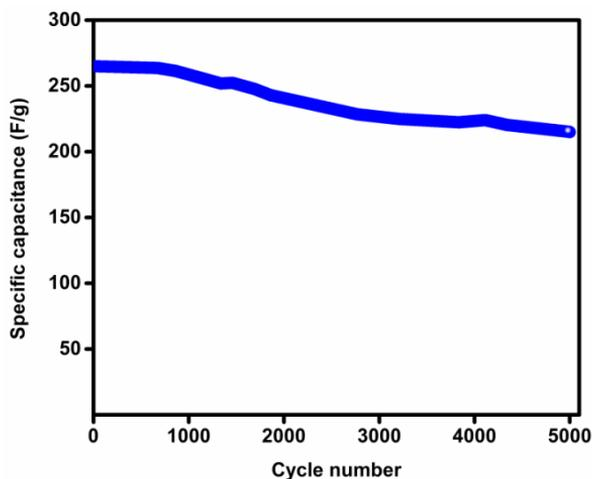
Fig. 10. Cycling stability of  $\text{Li}_4\text{Ti}_5\text{O}_{12}$  as electrode
