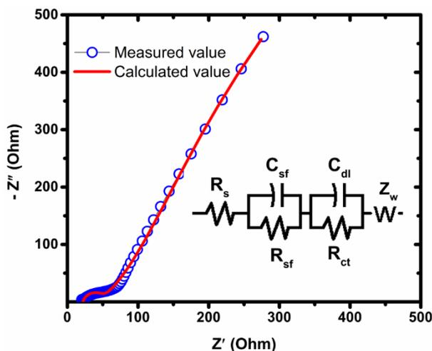
Fig. 9. Nyquist plot of nanocrystalline  $\text{Li}_4\text{Ti}_5\text{O}_{12}$  as electrode
