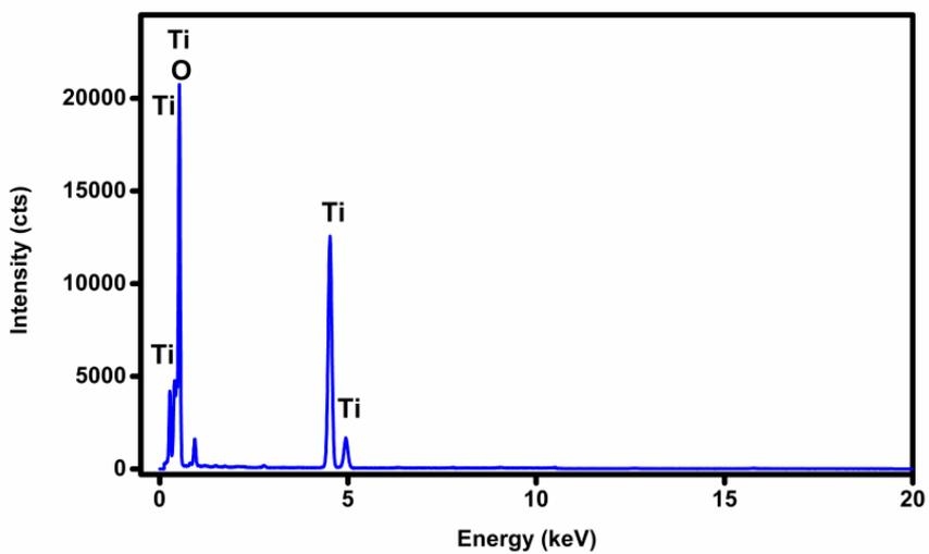
Fig. 5. EDS spectrum of  $\text{Li}_4\text{Ti}_5\text{O}_{12}$
