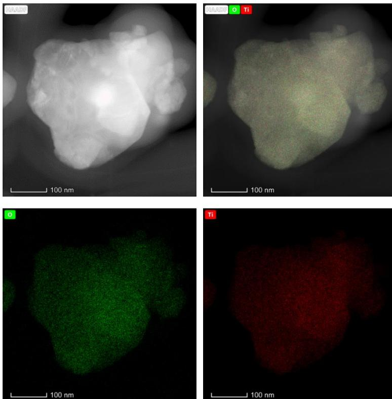
**Fig. 6.** Elemental mapping of  $\text{Li}_4\text{Ti}_5\text{O}_{12}$
