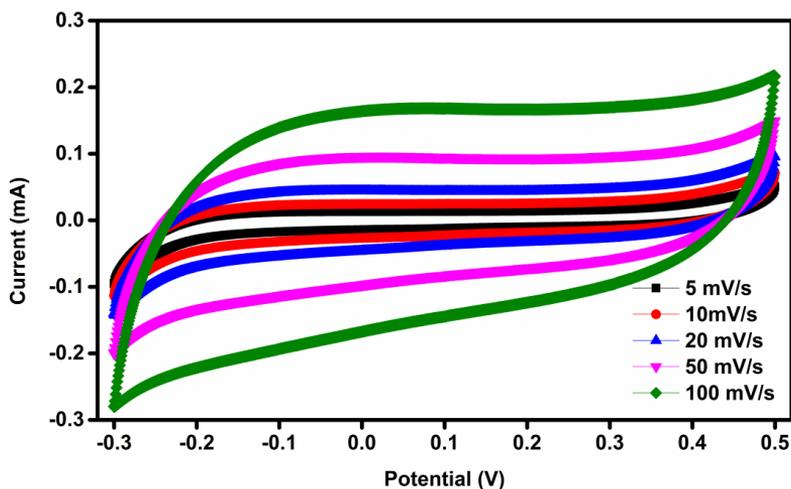
Fig. 7. Cyclic voltammograms of  $\text{Li}_4\text{Ti}_5\text{O}_{12}$  electrode recorded at different scan rates
