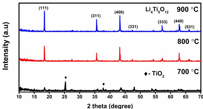
Fig. 1. XRD patterns of  $\text{Li}_4\text{Ti}_5\text{O}_{12}$  sintered at different temperatures
