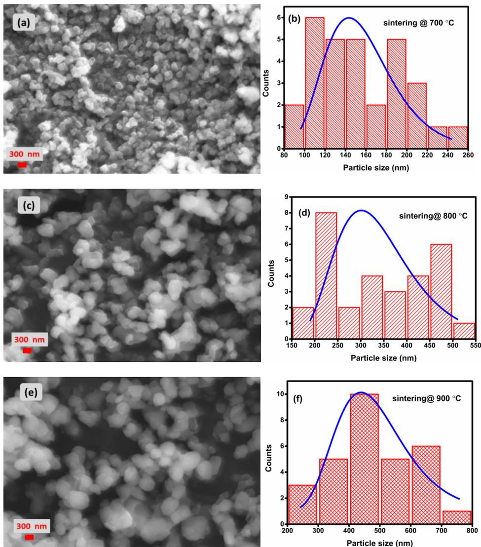
**Fig. 3.** Microstructural analysis and particle size distribution: a), c), e) SEM images of  $\text{Li}_4\text{Ti}_5\text{O}_{12}$  (sintered at 700 °C, 800 °C and 900 °C); b), d), f) their resultant statistical histogram for particle size distribution
