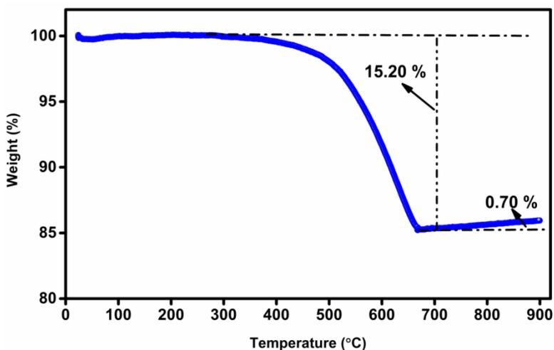
Fig. 2. TG analysis graph of  $\text{Li}_4\text{Ti}_5\text{O}_{12}$
