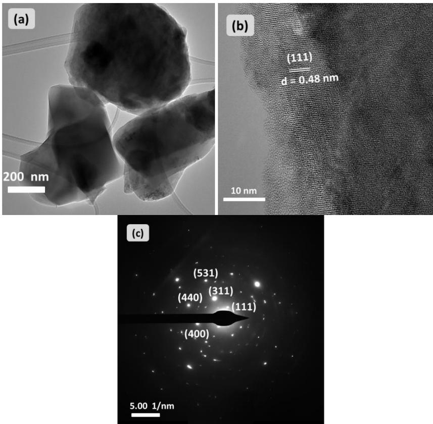
Fig. 4. Microstructural analysis: a), b) HRTEM images; c) SAED pattern of  $\text{Li}_4\text{Ti}_5\text{O}_{12}$
