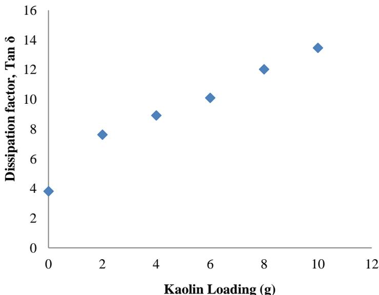
**Fig. 6.** Variation of the dissipation factor of polyester/metakaolin composite with kaolin loading at 20 Hz.
