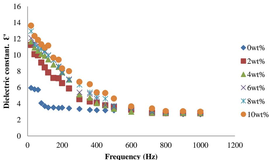
**Fig. 3.** Polyester/metakaolin composite's dielectric constant variation with frequency
