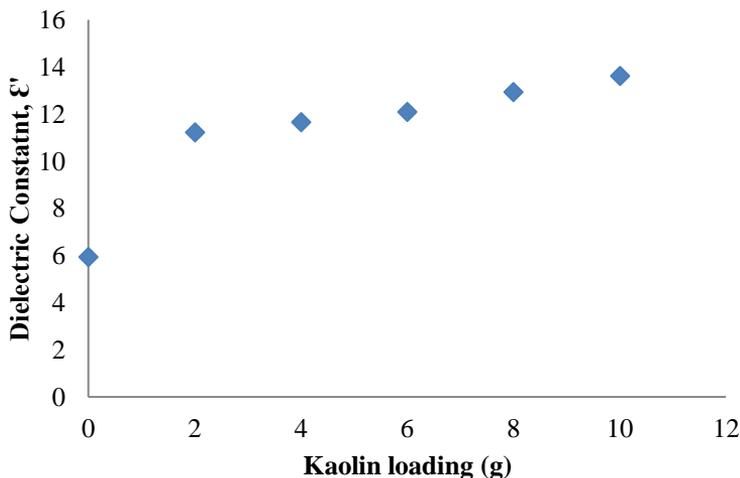
Fig. 4. Variation of the dielectric constant of polyester/metakaolin composite with kaolin loading at 20Hz.
