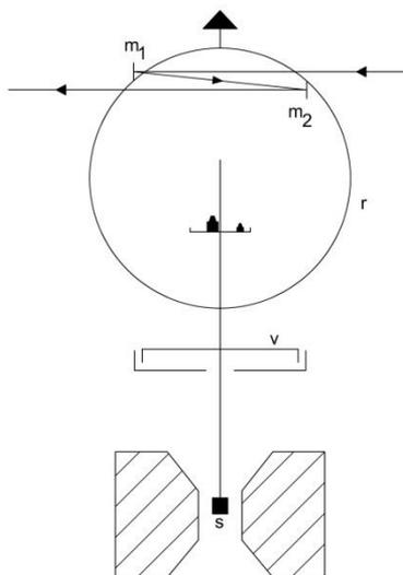
Fig. 1. Schematic representation of Sucksmith's type magnetic balance [17]
