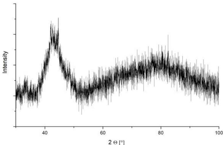
Fig. 4. Diffractometer of  $\text{Fe}_{60}\text{Co}_{10}\text{Y}_8\text{Ni}_2\text{B}_{20}$
