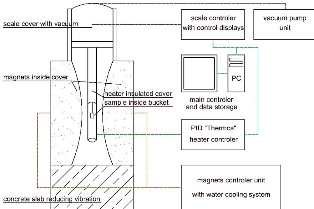
Fig. 2. Schematic representation of Farraday's magnetic balance setup
