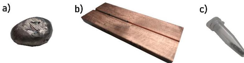
Fig. 3.  $Fe_{60}Co_{10}Y_8Ni_2B_{20}$  alloy produced: a) mechanically cleaned ingot, b) rod form amorphous alloy on the half of copper mold
