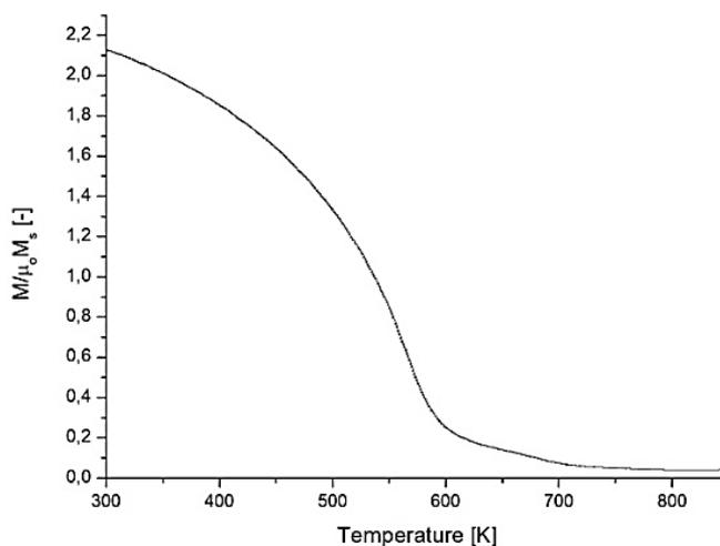
Fig. 5. Thermomagnetic curve obtained for  $\text{Fe}_{60}\text{Co}_{10}\text{Y}_8\text{Ni}_2\text{B}_{20}$
