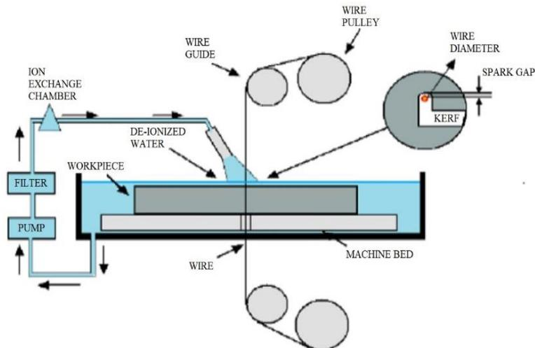
**Fig 1.** Schematic the WEDM process
