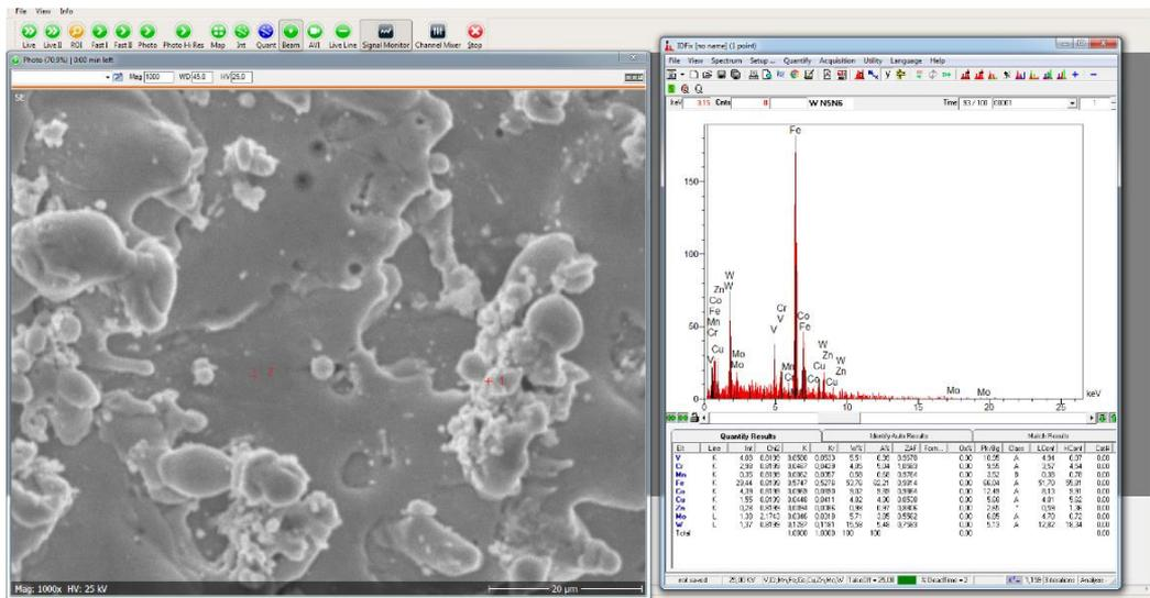
**Fig. 6.** Scanning electron micrograph and Energy Dispersive X-Ray Spectroscopy (EDS) after the first trim cut
