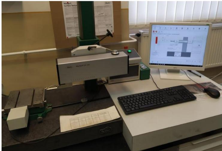
**Fig. 3.** MahrSurf GD120 roughness measuring machine
