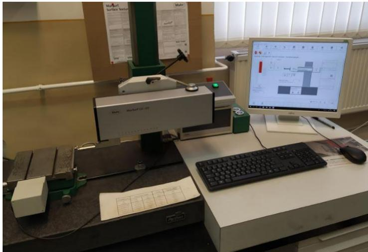
**Fig. 3.** MahrSurf GD120 roughness measuring machine
