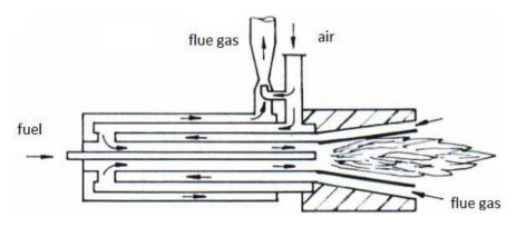
Fig. 3. Schematic diagram of the self-contained recovery burner
