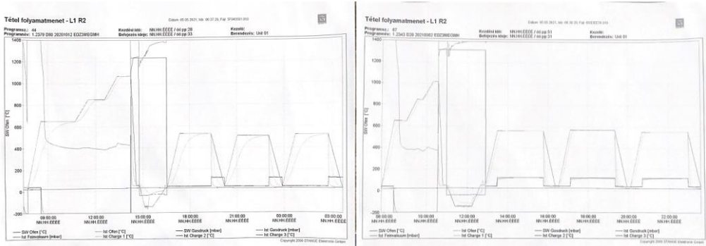
Fig. 5. The heat treatment diagram of the steel grades D2, respectively H11
