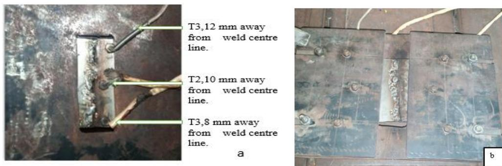
**Fig. 3.** The specimen showed: a) three k-type thermocouples planted at different points of interest away from b) the weld centreline for faces
