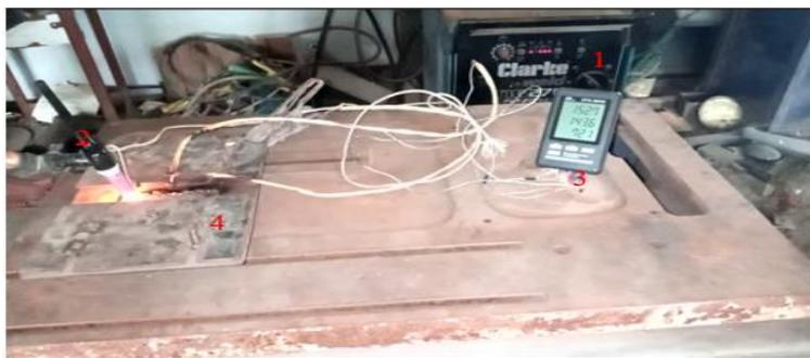
**Fig. 2.** Typical experimental procedure: 1-welding machine; 2-TIG torch; 3-Datalogger Datalogger with type K thermocouples –3 channel; 4-track
