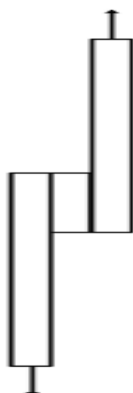
Fig. 5. a) Schematic lap shear test sample
