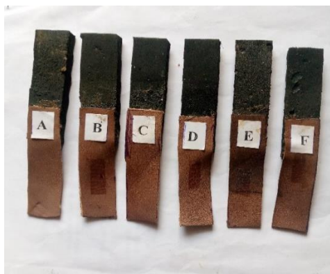
Fig. 5. d) Lap shear test samples of rubber to the leather outsole to insole material
