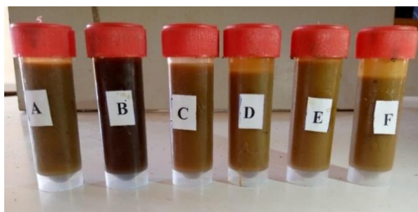
Fig. 3. Natural rubber base adhesive produced using mechanical mastication and chemical peptizer
