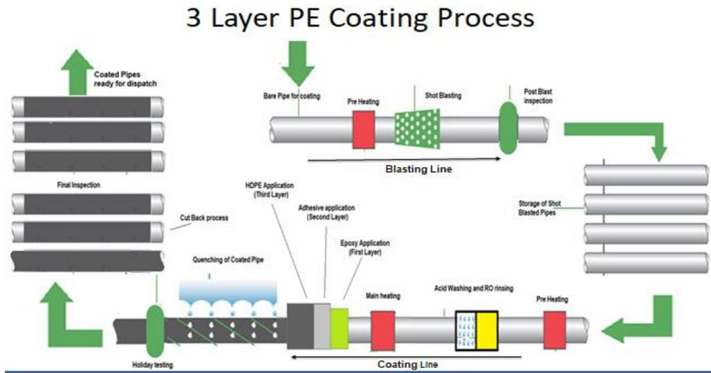
Fig. 1. Three layer polyethylene coating process utilized
