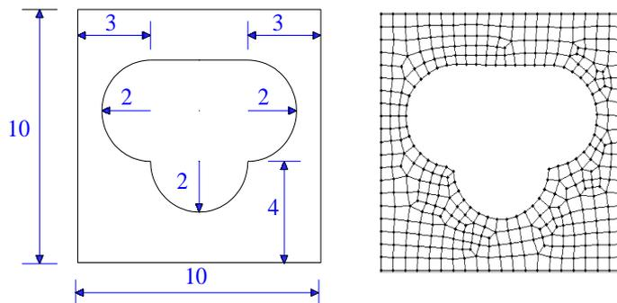
**Fig 5.** The functionally graded porous plate with complex cut-out II: Geometry properties, 318 quadrilateral elements
