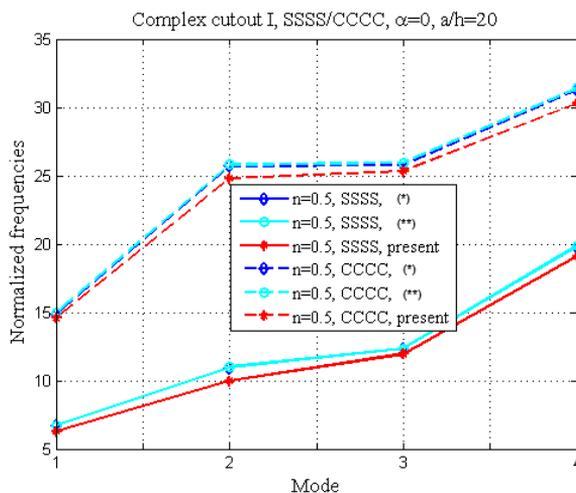
**Fig 3.** Comparison of the first four normalized frequencies of functionally graded porous plate with  $\alpha = 0, n = 0.5$  and  $a/h = 20$
