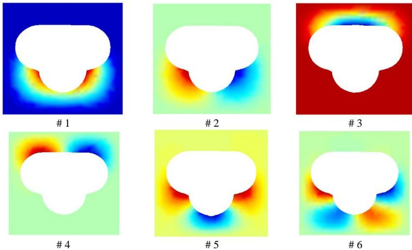
**Fig 7.** The first six mode shapes of functionally graded porous plate with complex cut-out II,  $a/h = 20, n = 1, \alpha = 0.4$ , even porosity and CCCC.
