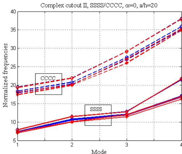
**Fig 6.** Comparison of the first four normalized frequencies of functionally graded porous plate with  $\alpha = 0$ ,  $n = 0, 0.5$  &  $1$  and  $a/h = 20$
