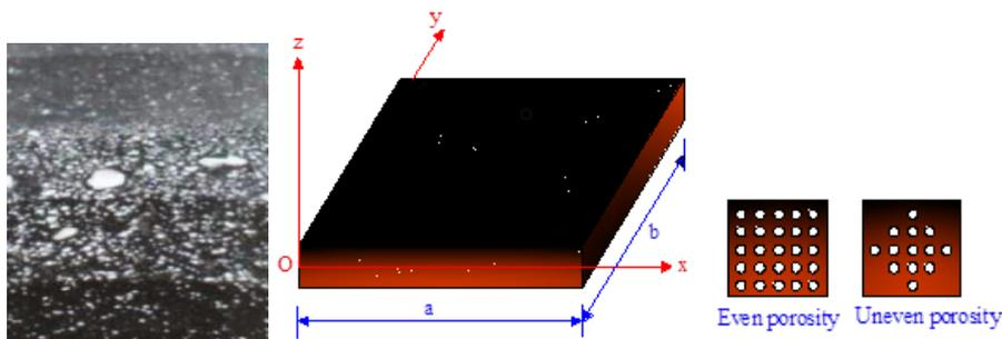
**Fig 1.** The functionally graded porous plate with both kinds of porosity [22]
