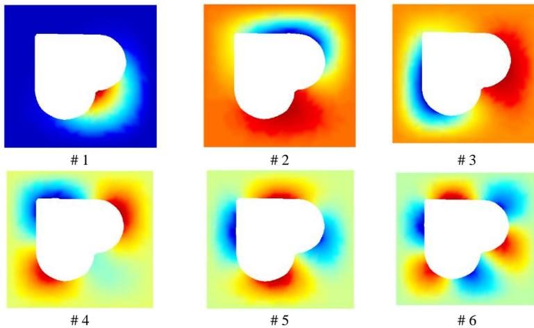
**Fig 4.** The first six mode shapes of functionally graded porous plate with complex cut-out I,  $a/h = 20$ ,  $n = 0$ ,  $\alpha = 0.4$ , even porosity and CCCC
