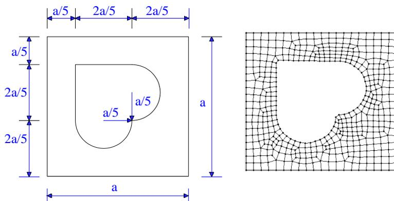
Fig 2. The functionally graded porous plate with complex cut-out I: geometry properties, 425 quadrilateral elements
