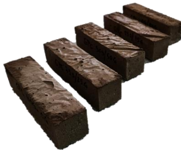
Fig. 5. Alkali activated fly-ash based geopolymer concrete samples with spent garnet used as sand replacement
