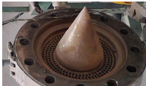
Fig. 1. Corroded tool, used during recycling of PVC
