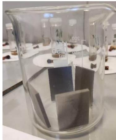
Fig. 5. Samples before submerging in the FeCl 3 solution
