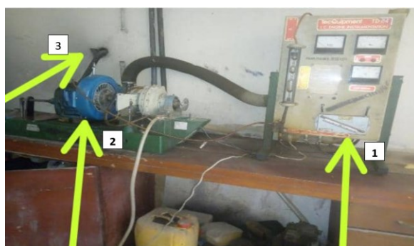
Fig. 1. F165 Diesel engine test rig connected to TD114 IC engine instrumentation: 1 - TD114 IC engine instrumentation; 2 - F165 Diesel engine test rig; 3 - Exhaust pipe
