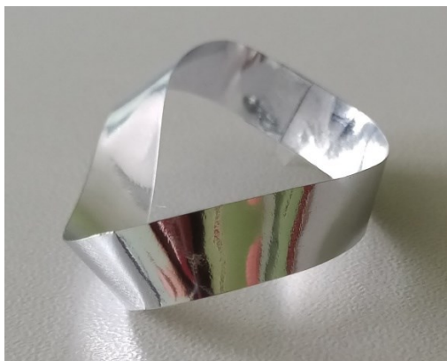
Fig. 2. The appearance on the Möbius strip resonator formed on the base of foiled polymer film
