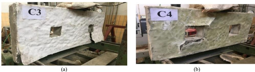
Fig. 8. De-lamination and rupture of beams with square openings a) 100mm and b) 160mm
