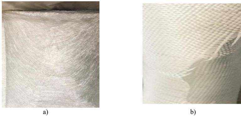
Fig. 1. Samples of GFRP a) mat fiber glass b) weaved fiber glass
