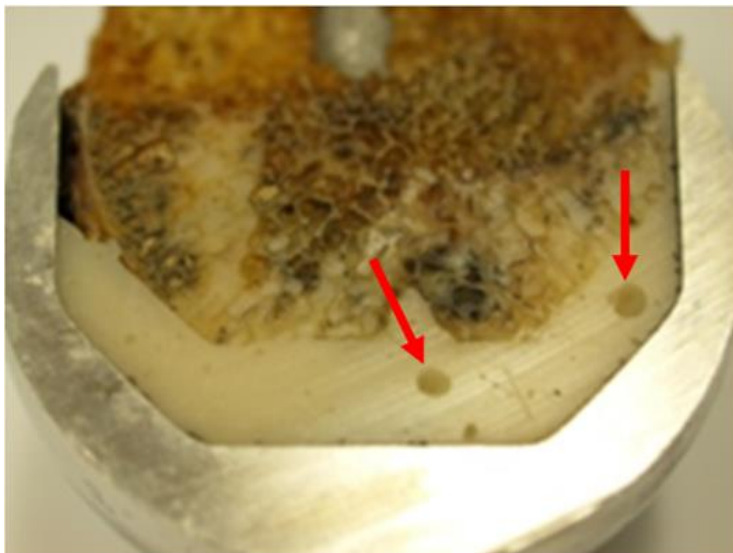
Fig. 2. Air bubbles formed in the cement mantle
