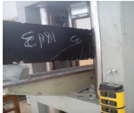
Fig. 8. Test setup with one-point loading
