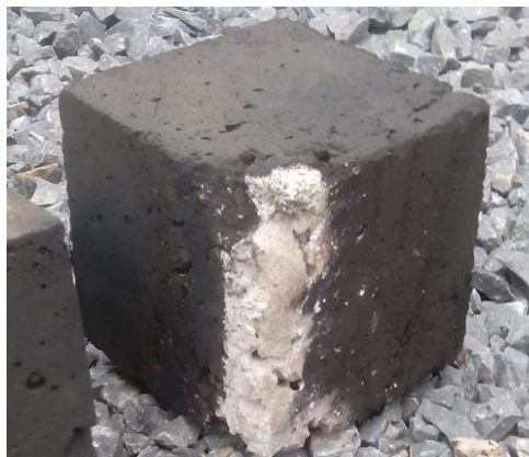
Fig. 5. Excessive burning of concrete cube
