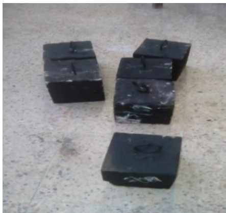
Fig. 4. Burnt and cooled concrete cubes
