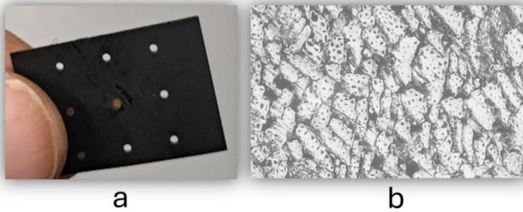
Fig. 5. (a) Cross-sectional plate filled with fibre cross-section, (b) Digital image of the fibre cross-sections.
