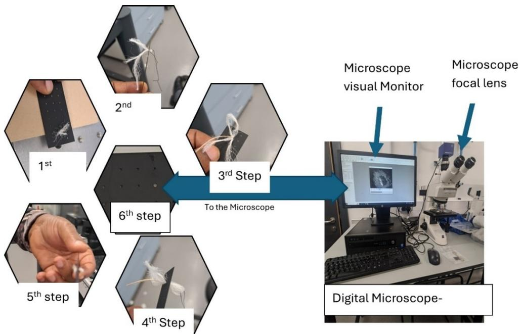
**Fig. 3.** Complete illustration of how to prepare and measure the cross-sectional areas of the jute fibre and yarn using a digital microscope measuring tools
