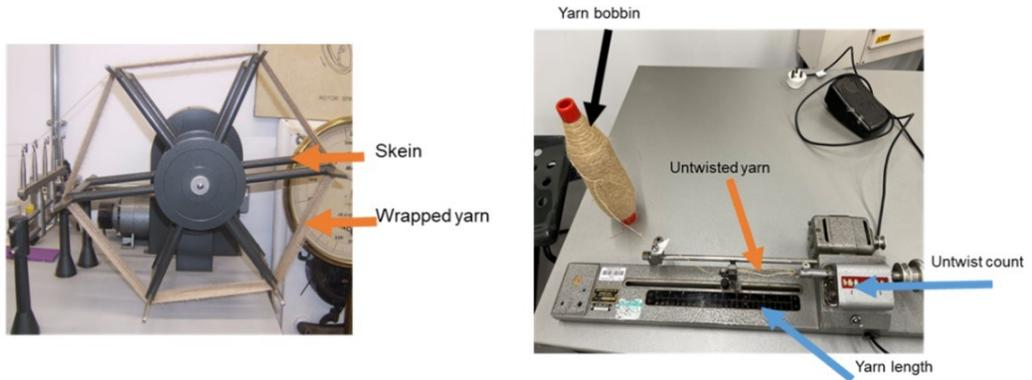
Fig. 1. Skein and twist metre
