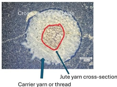
Fig. 6. Typical example of the jute yarn cross section obtained from Digital Microscope against the carrier yarn
