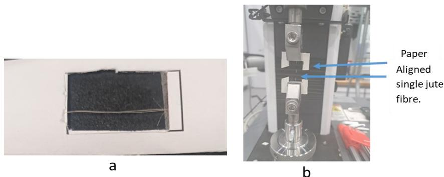
Fig. 7. Instron Universal Tensile Test Machine Setup for Fibre Testing
