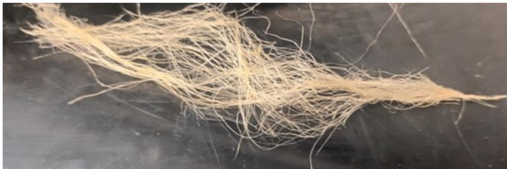
**Fig. 4.** Jute fibre extracted from jute yarn
