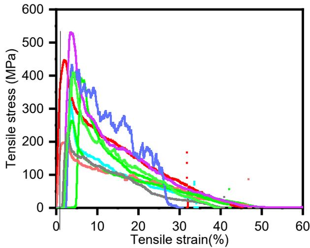
Fig. 8. Stress-strain graph of jute fibre tensile properties
