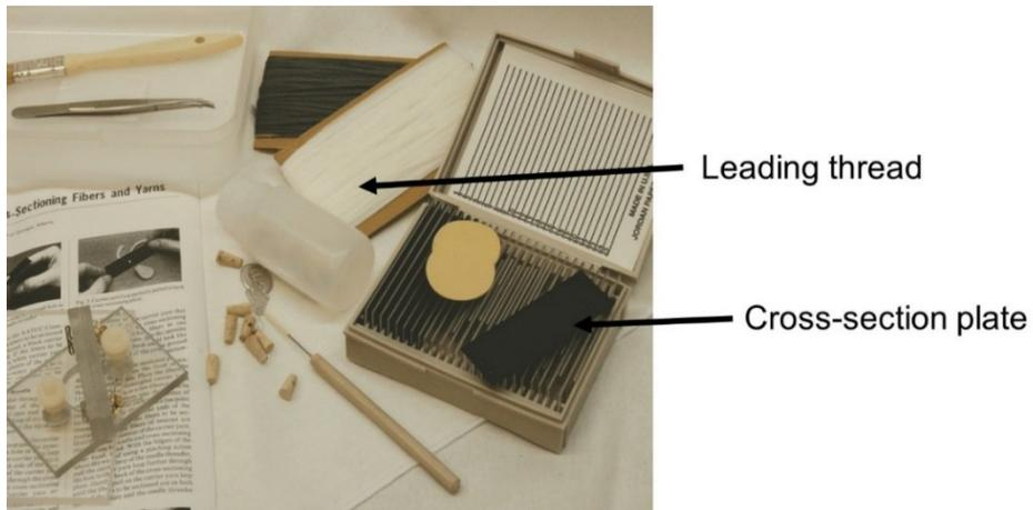
Fig. 2. Fibre and yarn cross-sectioning kit
