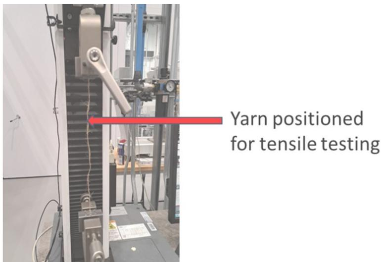
Fig. 9. Yarn tensile testing on an Instron Universal tensile testing machine.
