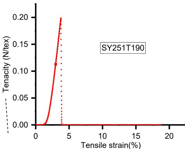
Fig. 10. A typical example of the yarn tenacity-strain graph
