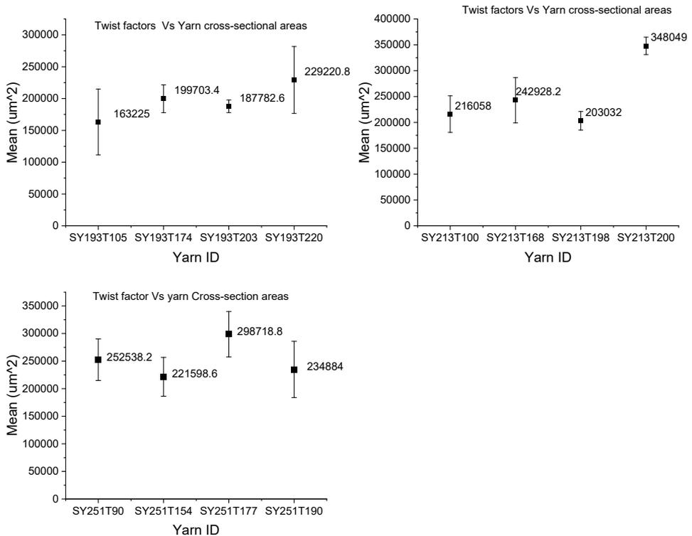
Fig. 10. The graphical impact of the twist factor on the cross-sectional area of yarns according to the linear densities.
