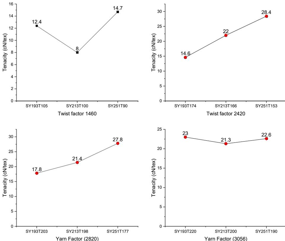
Fig. 11. Yarn tenacity versus twist factor when different yarn linear density is twisted with the same twist factor
