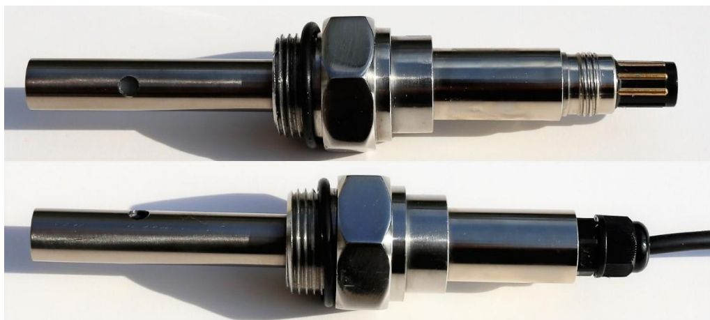
Fig. 5. The actual fabricated smart sensor / Fixed-cable type (bottom), detachable-cable type (top)
