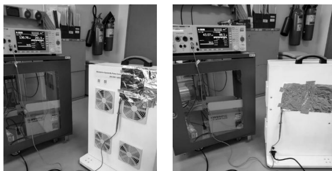
Fig. 6. Leakage current safety analysis test (IEC 60335-1) and total power analysis test is completed
