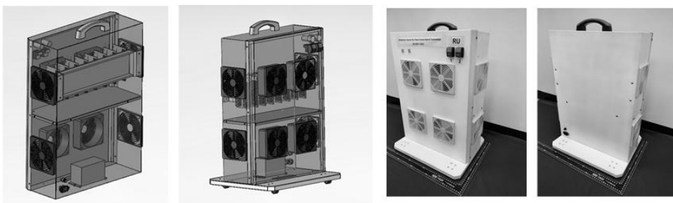
Fig. 4. Internal and external casing of the disinfection system using hybrid corona pulse technology. Compatible with circuit sizes, control systems, timers, and other systems
