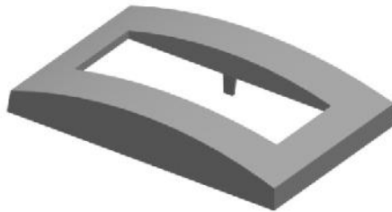
Fig. 1. The specimen of front panel housing.
