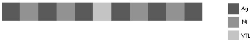
Fig. 1. Schematic of presented multilayer system. VTL - variable thickness layer.
