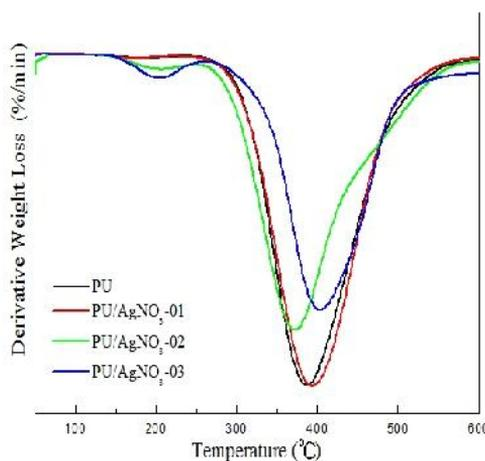
Fig. 3. DTG curves of the PU/AgNO<sub>3</sub>.
