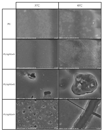
Fig. 7. SEM micrographs of the PU/AgNO3 with hydrolytic degradation for 12 d at 37°C and 45°C.
