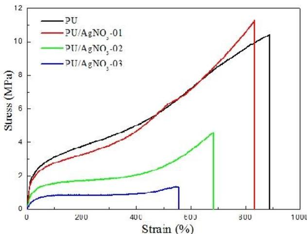
Fig. 5. Tensile properties of the PU/AgNO<sub>3</sub>.
