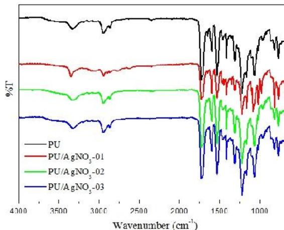
Fig. 1. FT-IR spectra of the PU/AgNO<sub>3</sub>
