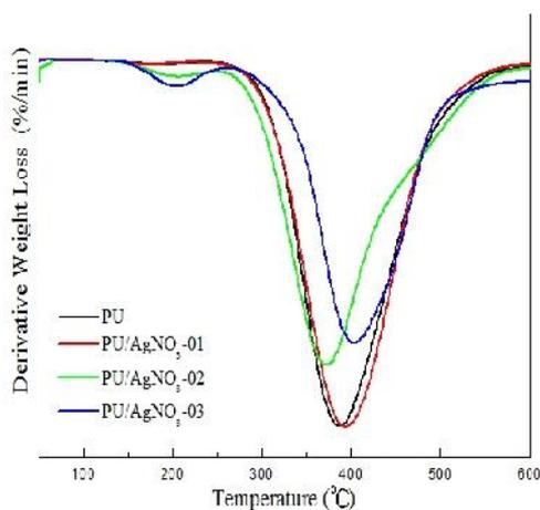
Fig. 3. DTG curves of the PU/AgNO<sub>3</sub>.
