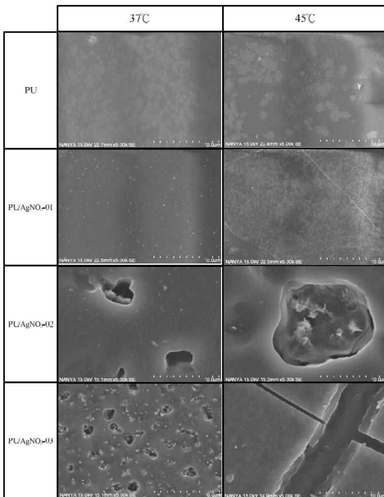
**Fig. 7.** SEM micrographs of the PU/AgNO<sub>3</sub> with hydrolytic degradation for 12 d at 37°C and 45°C.
