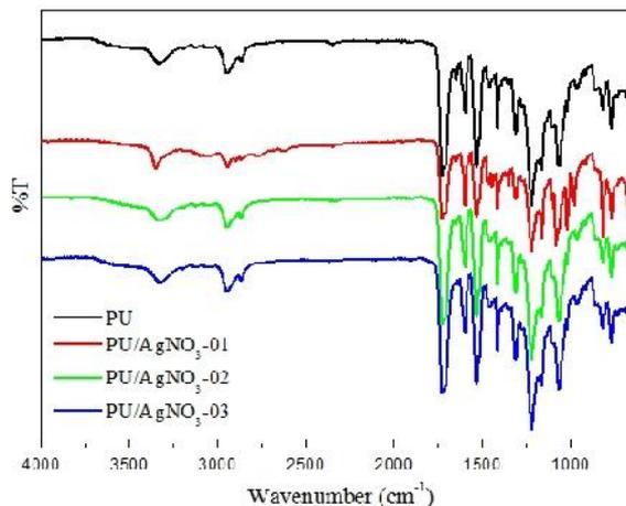
Fig. 1. FT-IR spectra of the PU/AgNO<sub>3</sub>
