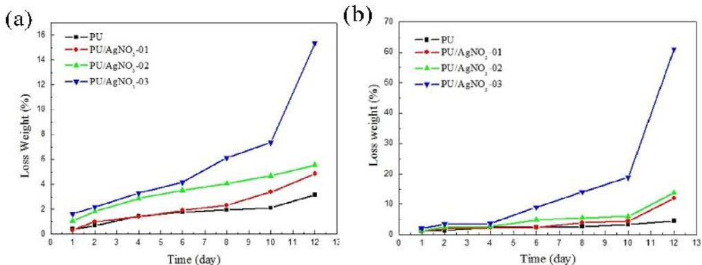
**Fig. 6.** Hydrolytic degradation results of the PU/AgNO<sub>3</sub>..
