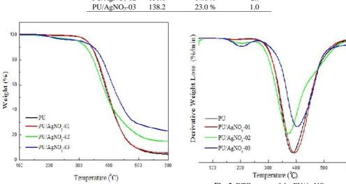
**Fig. 2.** TGA curves of the PU/AgNO<sub>3</sub>
