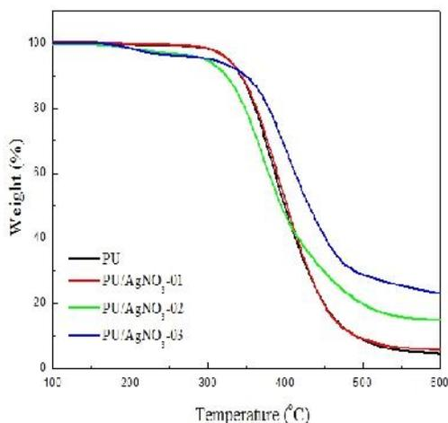
Fig. 2. TGA curves of the PU/AgNO<sub>3</sub>
