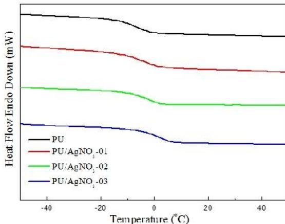
Fig. 4. DSC thermograms of the PU/AgNO<sub>3</sub>.
