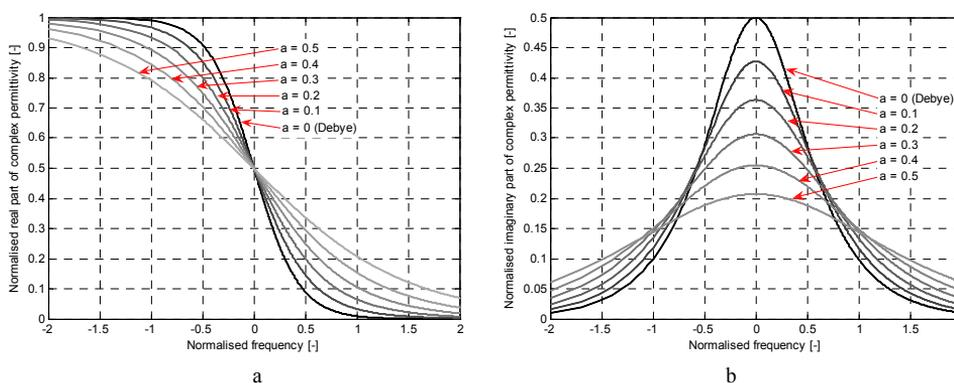
**Fig. 4.** The frequency dependence of (a) real and (b) imaginary part of complex permittivity for various values of distribution parameter  $\alpha$  in Cole – Cole equation.
