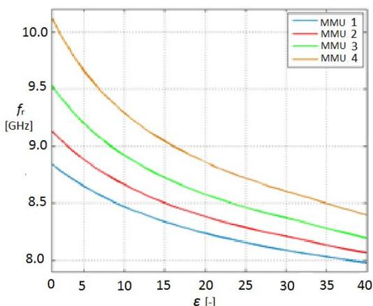
Fig. 9. Calibration curves for dielectric constant calculation.
