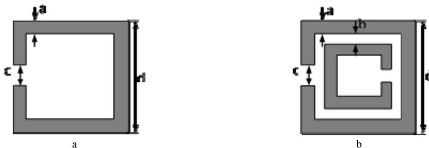
Fig. 1. Design of metamaterial unit for (a) single MMU and (b) double MMU.
