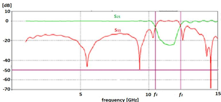
Fig. 7. The  $S_{11}$  and  $S_{21}$  – parameters of band-stop filter characteristics for designed waveguide sensor.
