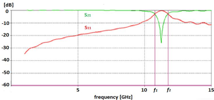
Fig. 6. The  $S_{11}$  and  $S_{21}$  – parameters of band-stop filter characteristics for one metamaterial unit.
