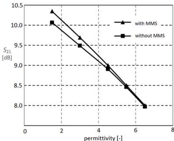
**Fig. 10.** Comparison of permittivity measurement with and without MMS inserted to the volume of classical waveguide sensor.
