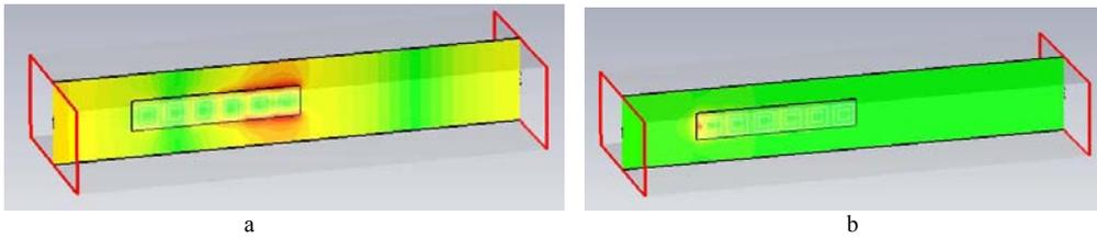
Fig. 5. The electromagnetic field distribution in waveguide sensor with metamaterial structure at (a) nonzero and (b) zero transmission.
