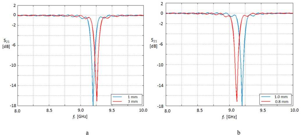
**Fig. 3.** Design of metamaterial unit; resonant frequency as a function of a) structures distance for double MMU, b) width of rectangle of MMU; transmission coefficient  $S_{21}$  as a function of resonant frequency.
