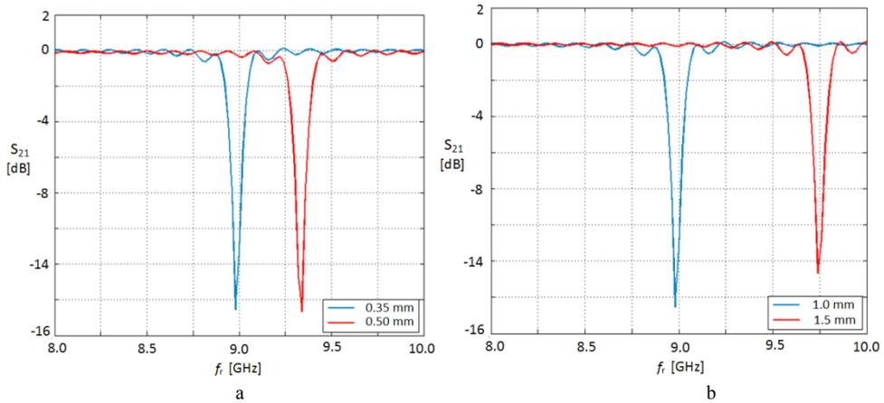
**Fig 2.** Design of MMU; resonant frequency as a function of width (dimension  $c$  and dimension  $b$ ) transmission coefficient  $S_{21}$  as a function of frequency.
