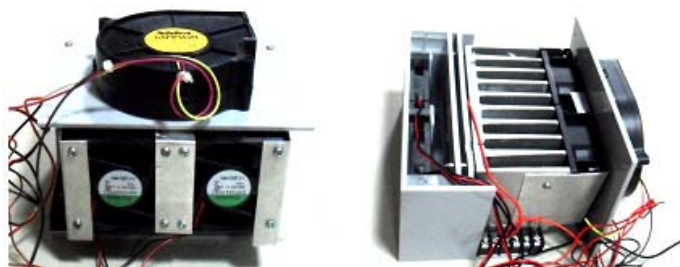
Fig. 7. Cool air production system by applied thermoelectric.
