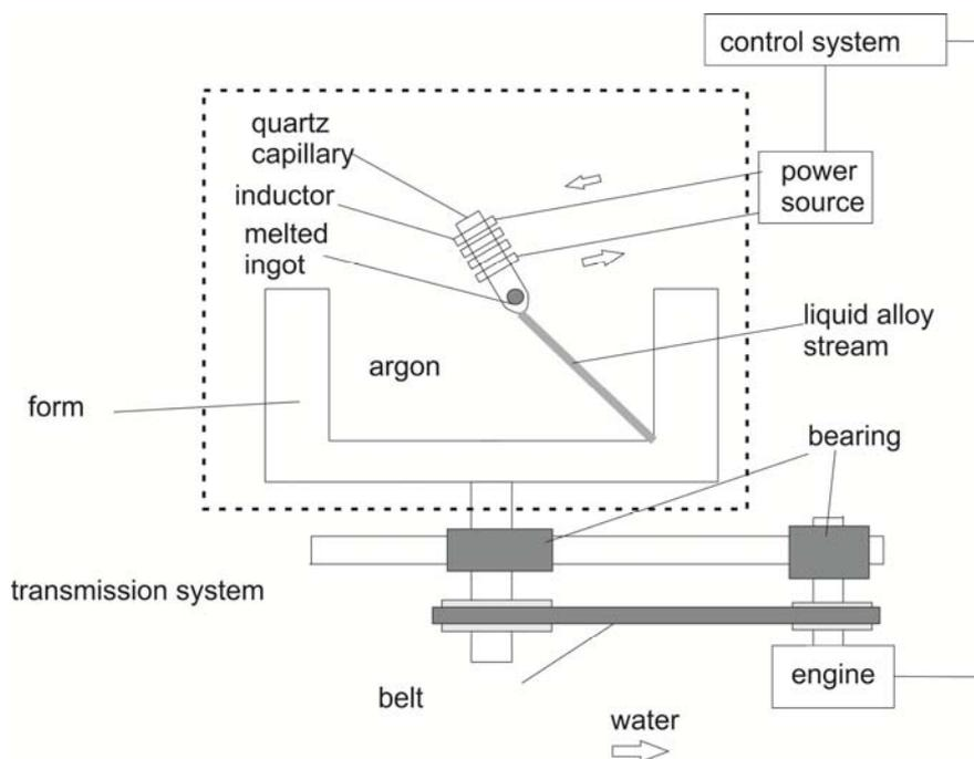
Fig. 3. Scheme production of amorphous materials by centrifugal method, side view
