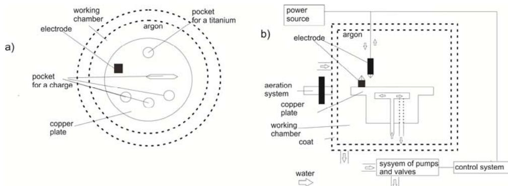
Fig. 1. Scheme of apparatus for making ingots using the arch method: a) top view, b) side view
