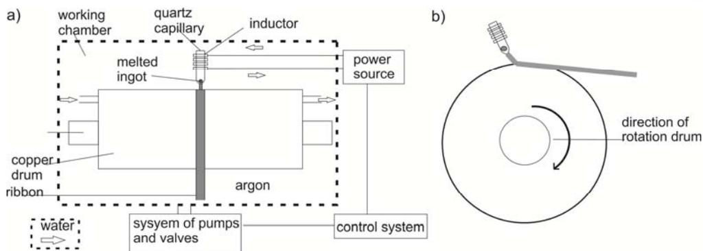
**Fig. 2.** Schematic production of amorphous materials by melt - spinning: a) Front view, b) Side view
