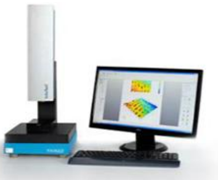
Fig.13. Solaris surface profilometer to capture erosion/corrosion image of the samples.
