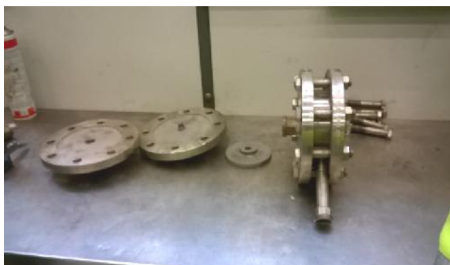
Fig.9. Detail of the mechanical components of the experimental equipment system (test unit holder).
