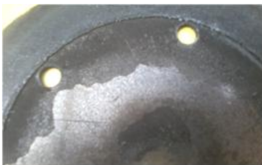
Fig.12. The un-coated test plates after 30 days of exposure to geothermal steam. Central area is much eroded minor scaling deposition from the geothermal steam.
