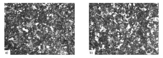
Fig.3. Microstructures of samples after low tempering heat treatment - magnitude: a) 200X; b) 100X.
