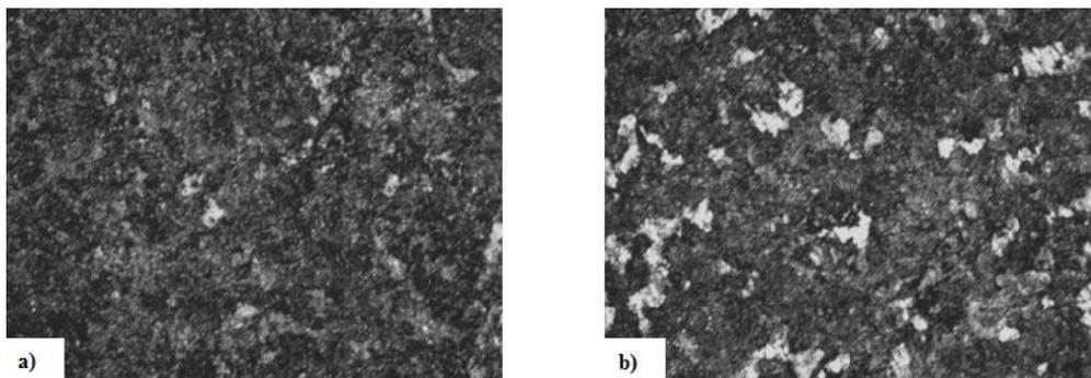
**Fig.1.** Microstructures of samples after annealing heat treatment - magnitude: a) 200X; b) 100X.
