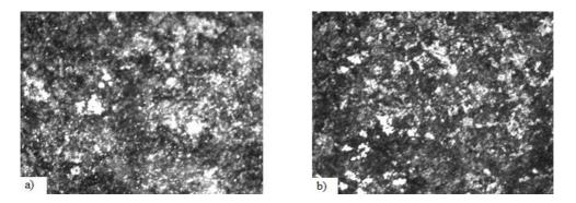
Fig.2. Microstructures of samples after martensitic quenching heat treatment - magnitude: a) 200X; b) 100X.
