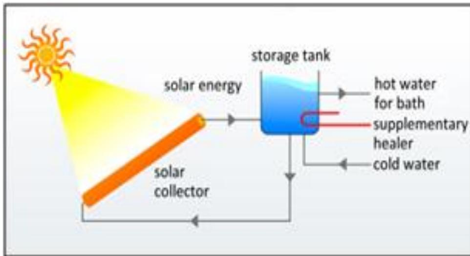
**Fig. 1.** Natural cycle type of solar water heater [8]
