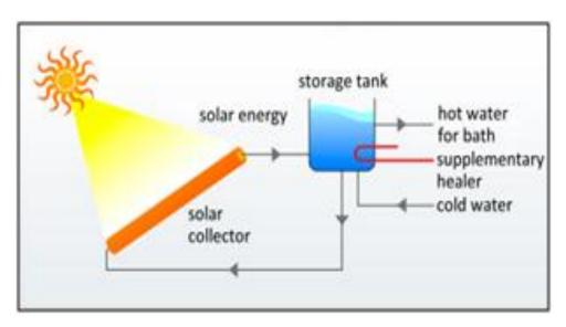
Fig. 1. Natural cycle type of solar water heater [8]
