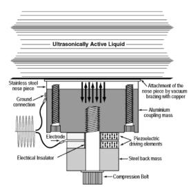
Fig. 3. Piezoelectric Transducer
