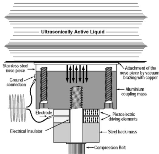
Fig. 3. Piezoelectric Transducer
