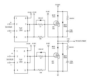
Fig. 5. Gate drive circuit
