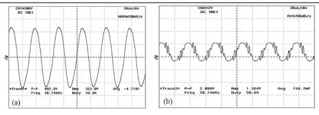
Fig. 9. (a) High frequency transformer output signal with probe x 100 and (b) High frequency transformer output current with current probe 10 mv/A.
