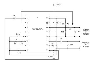
Fig. 4. Connecting the IC#SG3525A
