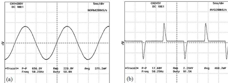
Fig. 8. (a) System input voltage signal while driving an ultrasonics transducer using probe x 100 and (b) Signal input current of the system while driving an ultrasonic transducer using current probe 10 mv/A
