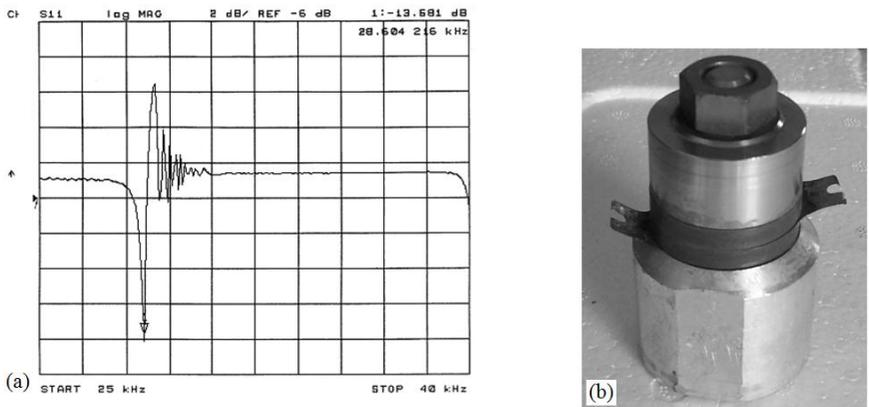
Fig. 7. (a) Ultrasonics frequency response graph transducer and (b) Ultrasonics transducer used in power 70 watts per head
