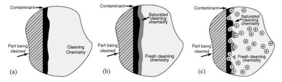
Fig.1. (a) Cleaning process, (b) Happen of transparent layers and (c) Destruction of the layer between the dirty surface and the solvent
