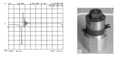
Fig. 7. (a) Ultrasonics frequency response graph transducer and (b) Ultrasonics transducer used in power 70 watts per head
