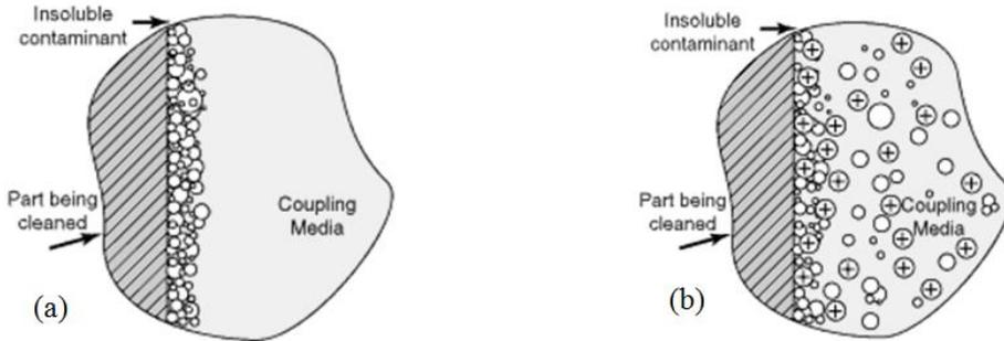
Fig. 2. (a) Particles of impurities attached and (b) Particles of impure impurities [1]
