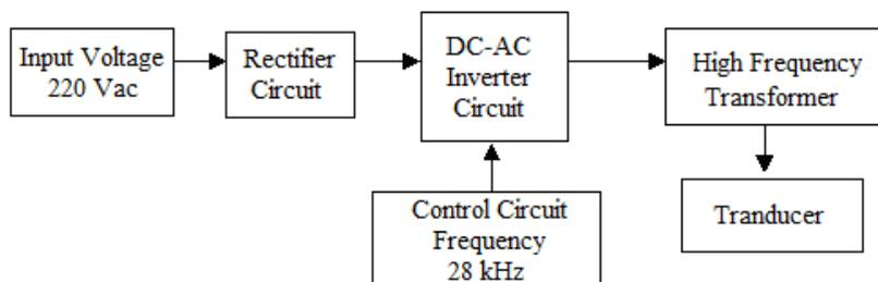
Fig. 6. Block diagram of high frequency high voltage switching power supply
