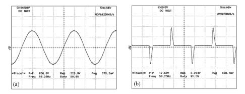
**Fig. 8.** (a) System input voltage signal while driving an ultrasonics transducer using probe x 100 and (b) Signal input current of the system while driving an ultrasonic transducer using current probe 10 mv/A
