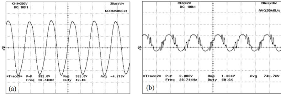
Fig. 9. (a) High frequency transformer output signal with probe x 100 and (b) High frequency transformer output current with current probe 10 mv/A.
