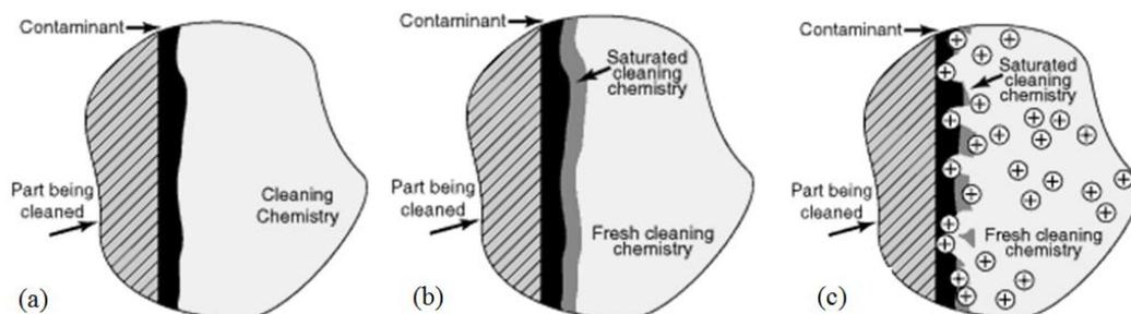
**Fig.1.** (a) Cleaning process, (b) Happen of transparent layers and (c) Destruction of the layer between the dirty surface and the solvent
