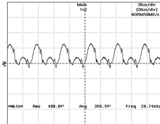
Fig. 10. High frequency transformer output power using Probe x 100 and current probe 10 mV/A.
