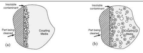
Fig. 2. (a) Particles of impurities attached and (b) Particles of impure impurities [1]
