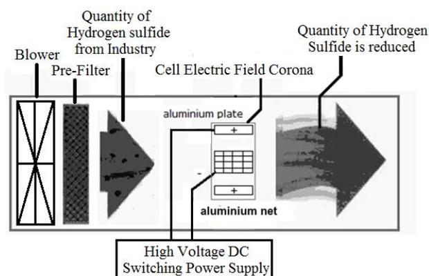
Fig. 1. The internal structure of the smell eliminator with cell electric field.
