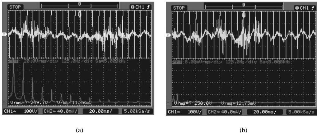
**Fig. 5.** (a) FFT signal of input current (before installation cool air production system) and (b) FFT signal of input current (after installation cool air production system)
