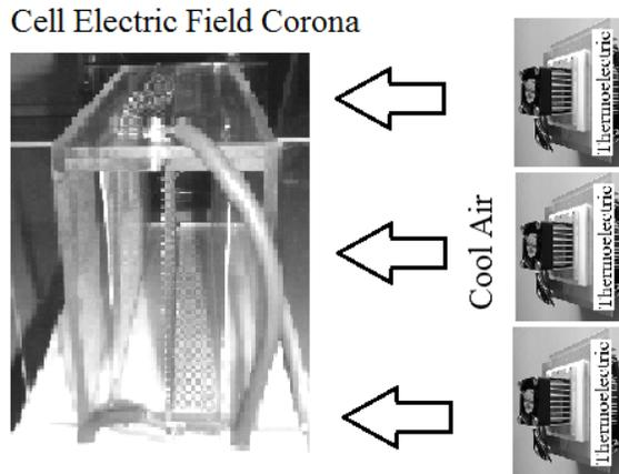
Fig. 4. Used cool air production from thermoelectric application for cell electric field corona.
