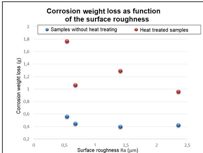
Fig. 7. Corrosion effected weight loss [12]
