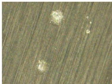
**Fig. 1.** Local corrosion form on the surface of stainless steel
