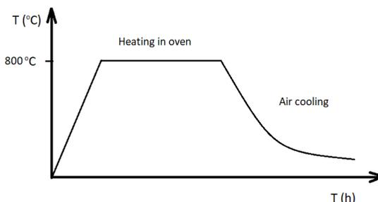
**Fig. 2.** Heat treatment of samples
