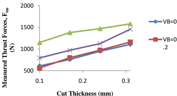
Fig. 3. Effect of cut thickness on measured thrust forces ( $F_{tm}$ ) at  $V=200$  m/min,  $\gamma = 0^\circ$
