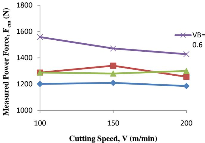
Fig. 4. Effect of cutting speed on measured power forces ( $F_{cm}$ ) at  $\gamma = 0^\circ$ ,  $t=0.17$  mm
