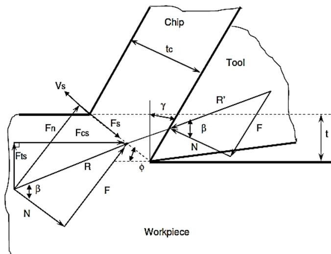
Fig. 1. Geometry of orthogonal cutting process
