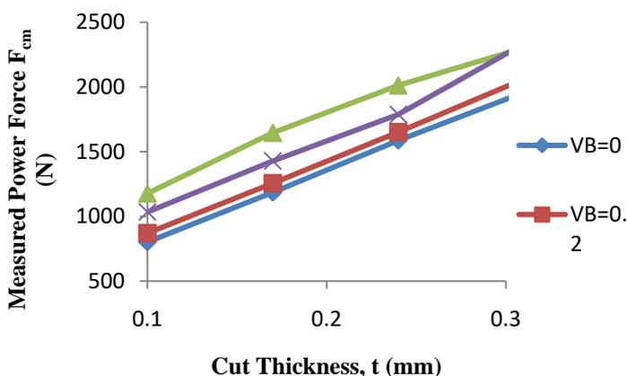
Fig. 2. Effect of cut thickness on measured power forces ( $F_{cm}$ ) at  $V=200$  m/min,  $\gamma = 0^\circ$
