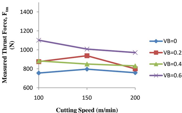
Fig. 5. Effect of cutting speed on measured thrust forces ( $F_{tm}$ ) at  $\gamma = 0^\circ$ ,  $t=0.17$  mm
