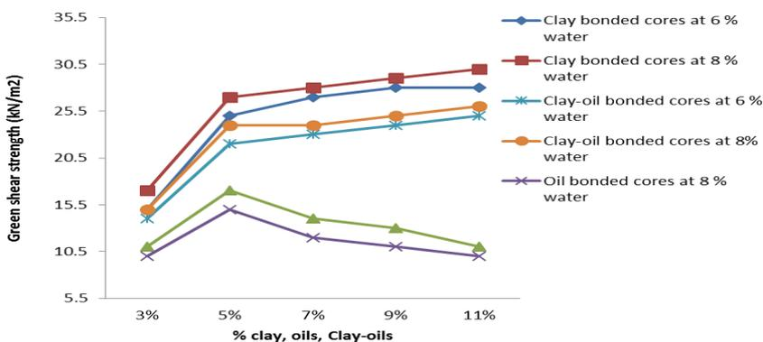
Fig. 5. Effect of percentage of orihi clay, jatropha-nigella sativa oils bonded cores on green shear strength at 6 and 8 % water
