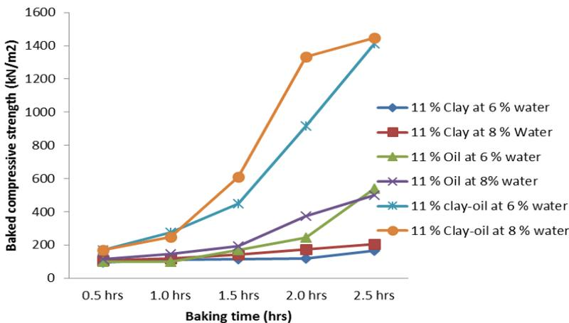
Fig. 4. Variation of baking time with baked compressive strength at 11 % for orihi clay, jatropha curcas-nigella sativa oil, and clay-oil bonded core at 6 and 8 % water at a baking temperature of 180 °c for a baking interval of 0.5-2.5 hours
