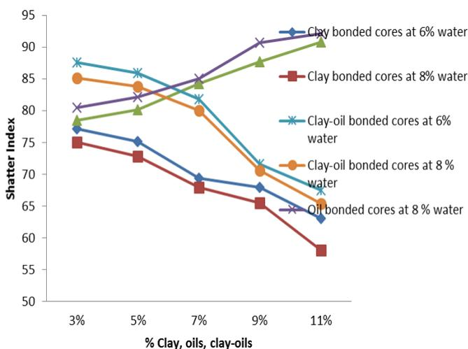
**Fig. 1.** Variation of orihi clay, *jatropha curcas-nigella sativa* oils, and clay-oil bonded cores on shatter index at 6 and 8 % water
