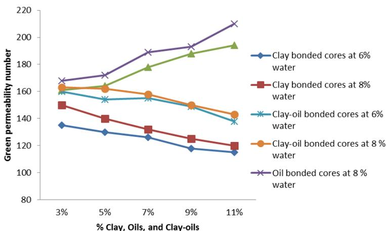
Fig. 2. Variation of orihi clay, jatropha curcas-nigella sativa oils, and clay-oil bonded cores on green permeability at 6 and 8 % water
