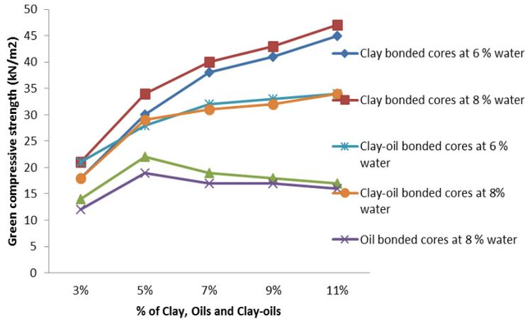
Fig. 3. Effect of orihi clay, jatropha-nigella sativa oil bonded cores on green compressive strength at 6 and 8 % water
