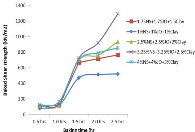
Fig. 6. Effect of baking time on baked shear strength at 8 % water on orihi clay, jatropha curcas-nigella sativa bonded core at baking temperature of 180 °c within a baking intervals of 0.5-2.5 hours
