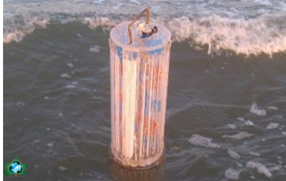
Fig. 10. In situ testing of the laboratory model - Off-shore complex for renewable energy production
