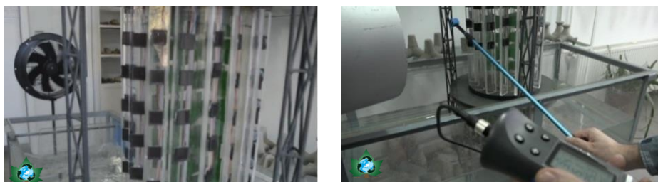
Fig. 13. Start-up of the aerial module and measuring the amount of air velocity that is directed to the laboratory model
