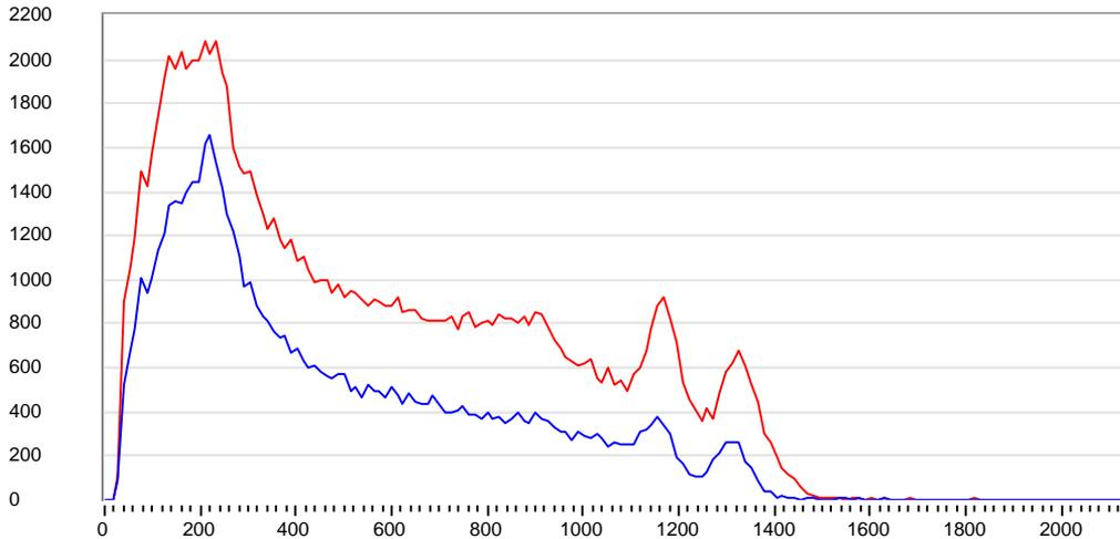
Fig. 2. Display gamma spectrometric two Co-60 sources
