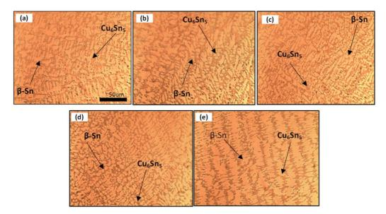
Fig. 1. Optical micrograph of the Sn-0.7Cu+xBi (x=0.0 wt.%, 0.50 wt.%, 1.00 wt.%, 1.50 wt.%, and 2.00 wt.%) on the bulk solder alloys
