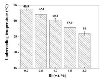
Fig. 3. Effect of Bi to undercooling temperature in Sn-0.7Cu solder alloy
