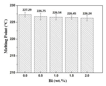
Fig. 2. Effect of Bi to melting temperature in Sn-0.7Cu solder alloy
