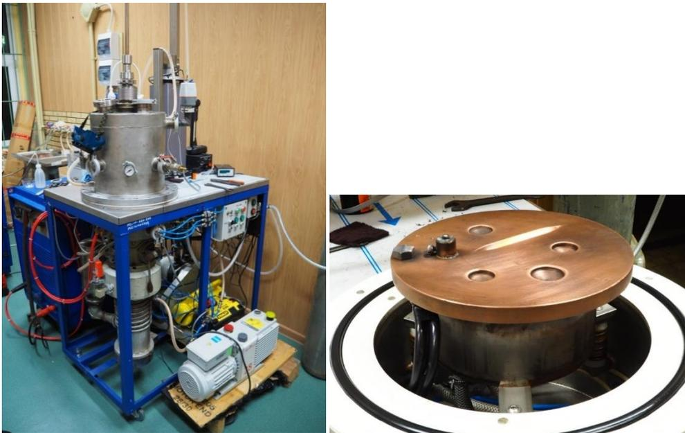
**Fig. 1.** Vacuum arc furnace
