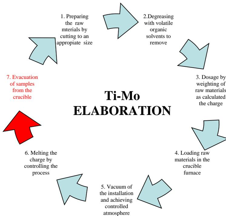
**Fig. 2.** Technological flow of Ti-Mo alloys
