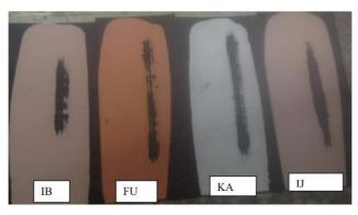
Fig. 1. The worn surfaces after wet abrasion testing on the paints samples
