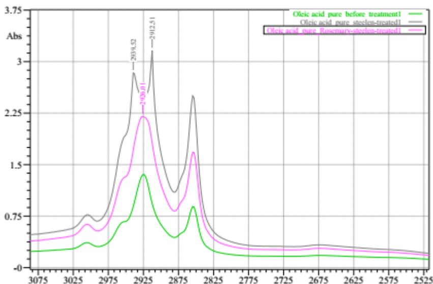
**Fig. 1.** FTIR Spectra of measured samples; red line oleic acid before treatment, pink line is for oleic acid mixed with Rosemary and stainless steel (Cr-Ni), black line oleic acid with stainless steel (Cr-Ni)
