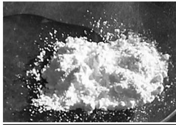
**Fig. 1.** Titanium dioxide powder physical appearance
