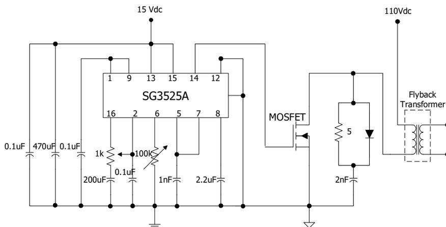
Fig. 2. High voltage power supply designed
