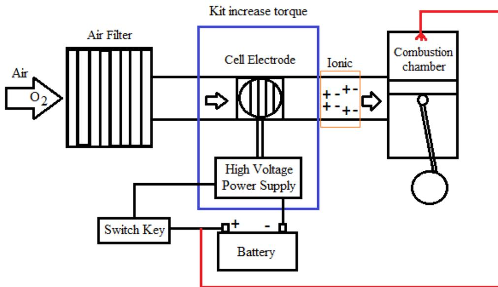
Fig. 1. Map of the installation of equipment kit for increasing torque of car designed
