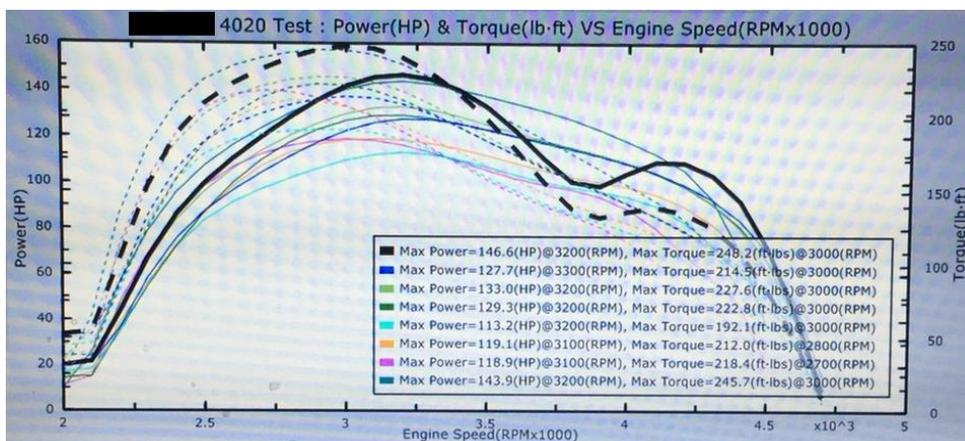
**Fig. 5.** Test results for torque measurements
