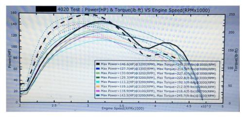
Fig. 5. Test results for torque measurements
