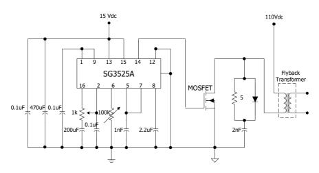
Fig. 2. High voltage power supply designed
