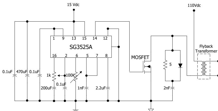
**Fig. 2.** High voltage power supply designed
