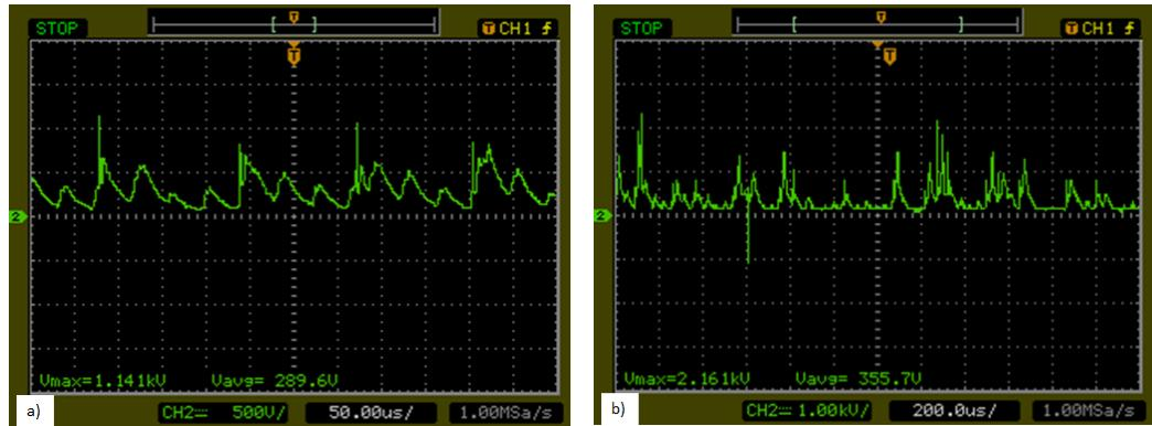
**Fig. 4.** (a) Output voltage high voltage signal ( $V_{OUT}$ ) of switching transformer is equal to  $1.14 \text{ kV}_p$  at duty cycle 10 % and (b) high voltage output signal ( $V_{OUT}$ ) of switching transformer is equal to  $2.16 \text{ kV}_p$  at duty cycle 20% while connecting the electrode
