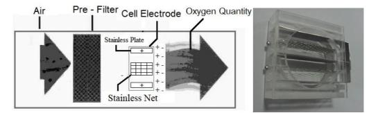
Fig. 3. Cell electrode for equipment kit for increasing torque in the diesel engine
