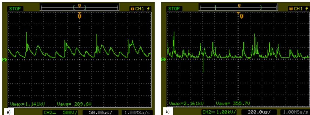
**Fig. 4.** (a) Output voltage high voltage signal ( $V_{OUT}$ ) of switching transformer is equal to 1.14 kV<sub>p</sub> at duty cycle 10 % and (b) high voltage output signal ( $V_{OUT}$ ) of switching transformer is equal to 2.16 kV<sub>p</sub> at duty cycle 20% while connecting the electrode
