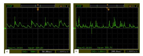
Fig. 4. (a) Output voltage high voltage signal ( $V_{OUT}$ ) of switching transformer is equal to 1.14 kV<sub>p</sub> at duty cycle 10 % and (b) high voltage output signal ( $V_{OUT}$ ) of switching transformer is equal to 2.16 kV<sub>p</sub> at duty cycle 20% while connecting the electrode
