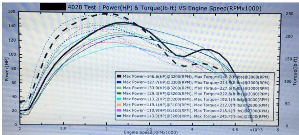
**Fig. 5.** Test results for torque measurements
