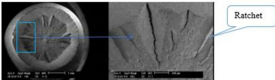
Fig. 11. Ratcheting marks, indicated by the arrows, in an CK35 shaft fractured by tensile
