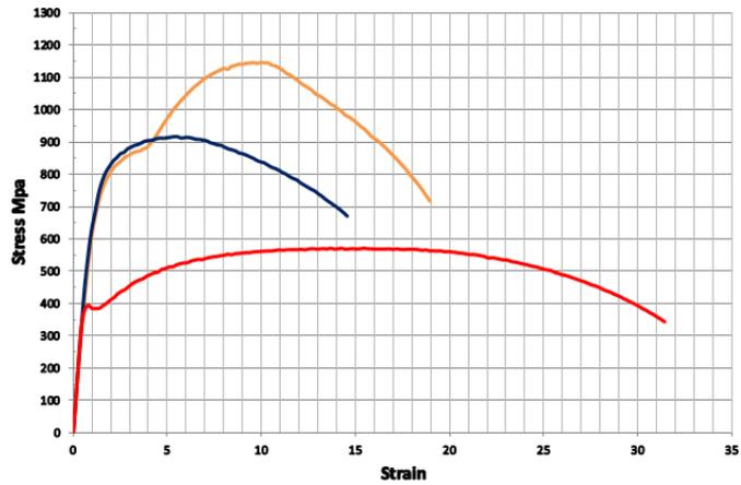
Fig. 4. Engineering stress–strain curves for CK35 at different quenching media.
