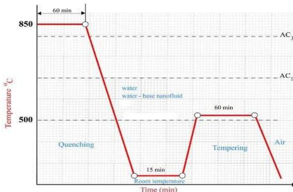
**Fig. 3.** Schematic illustration of heat treatment cycle used in this study.
