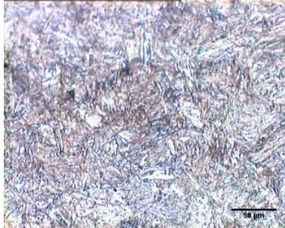
**Fig. 7.** Optical micrograph of microstructure of CK35 after quenching at water and tempering
