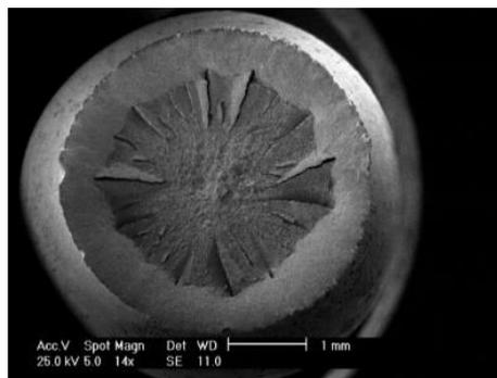
**Fig. 8.** Ductile fracture showing the typical cup-cone geometry at CK35 steel after quenching and tempering
